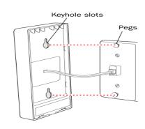
**3.** Connect the telephone cord to the phone jack located on the front of the mounted filter.
